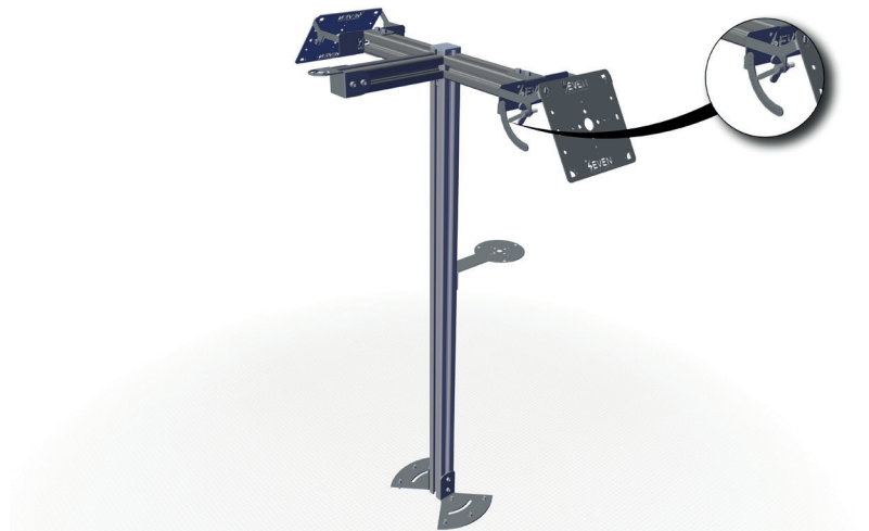
Figure 6 – Protractor on the Mounting Structure
