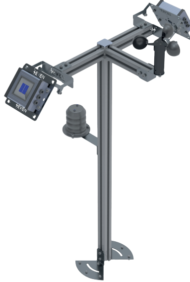
Figure 1 – Dual Orientations Irradiance Sensor
