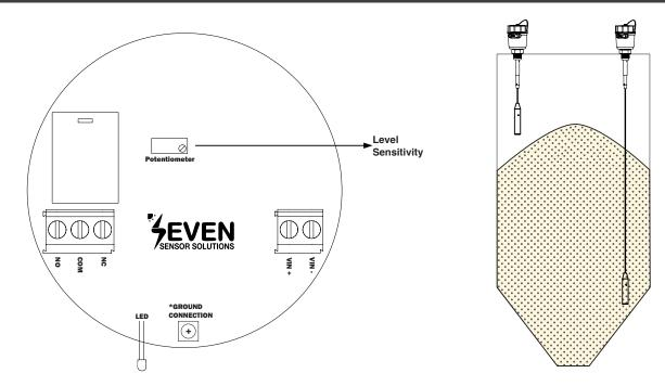
When the solid material in the silo, tank, or bunker is below the set level of the capacitive silo sensor or when these storage units are empty, the COM–NC connection becomes active, and the warning light starts flashing.
