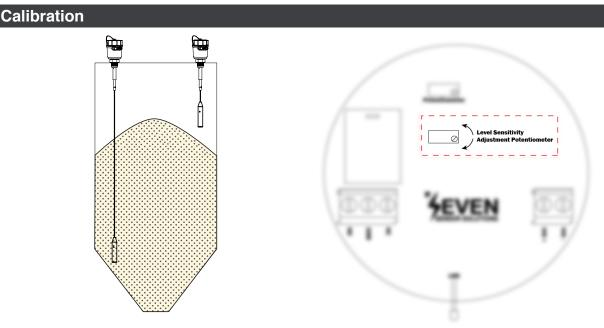
For product calibration, fill the silo/tank/bunker to the desired trigger level, then adjust the calibration potentiometer on the product until the LED light remains steady. The point at which the LED light remains steady is the calibration point.
