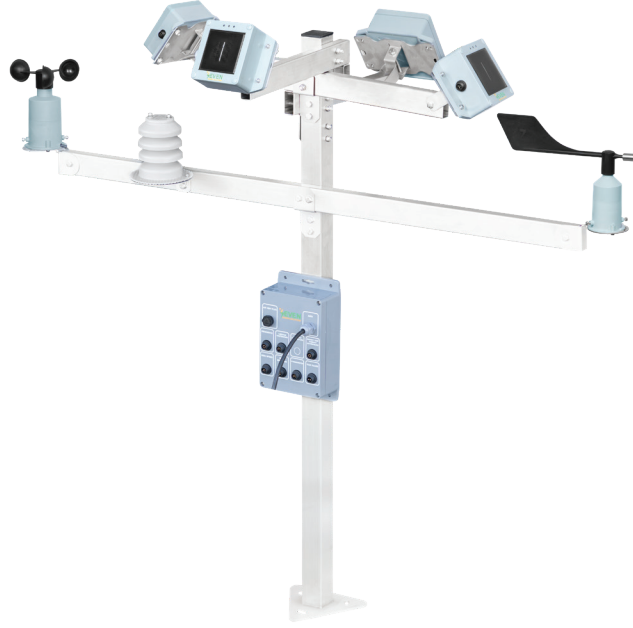
Figure 1 – Four-directional mounting structure
