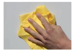
Clean the module's rear surface of oil and dust by using lint-free wipes dampened with a 70 % solution of isopropyl alcohol in distilled water. Allow all cleaned surfaces to dry completely before proceeding.
