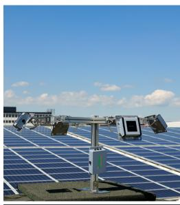
SEVEN Multi-Orientation Irradiance Sensor is part of the SEVEN meteorological sensor range, which includes professional and intelligent measurement sensors with a digital interface for environmental and industrial applications such as three or four orientation PV plants.
