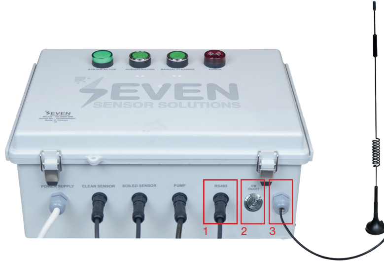
Figure 26 – Gateway Antenna Position
