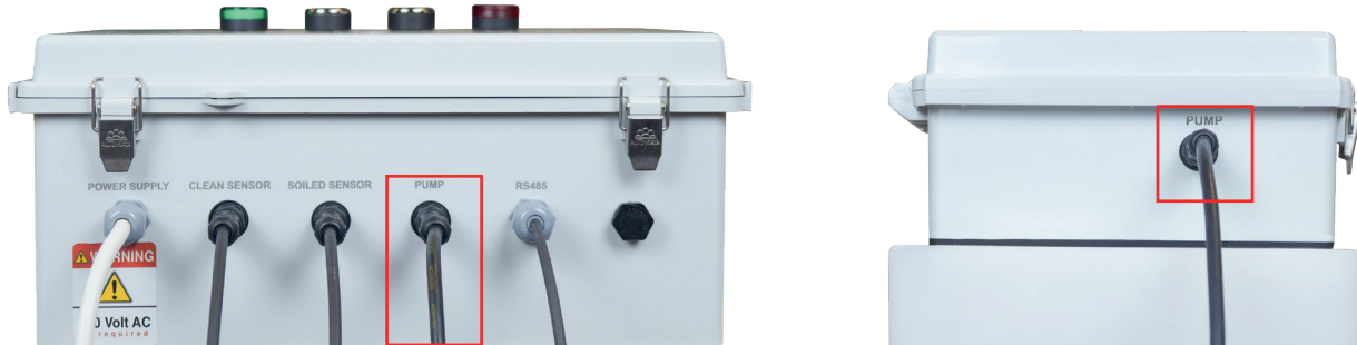
Figure 13 – Connection of the Water Pump Cable
