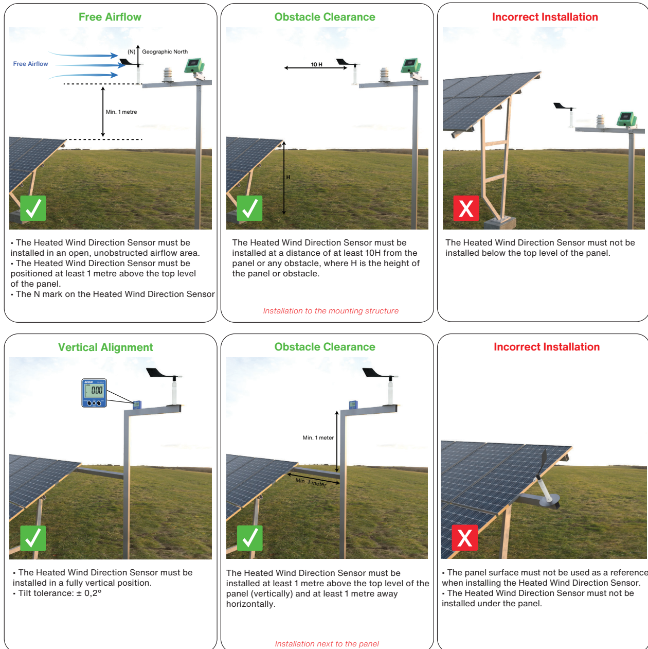
Figure 8 - Correct and Incorrect Field Installation
